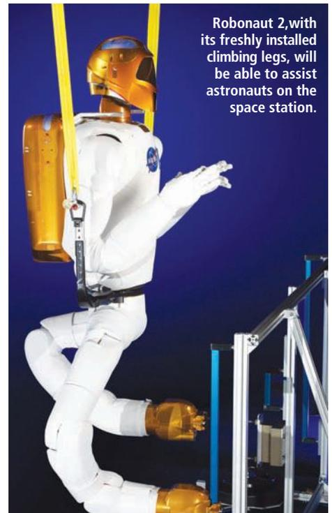
Robonaut 2, with its freshly installed climbing legs, will be able to assist astronauts on the space station.
